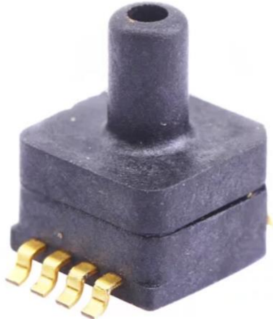
Figure 5.5 Pressure sensor in MEMS technology ( [14])
