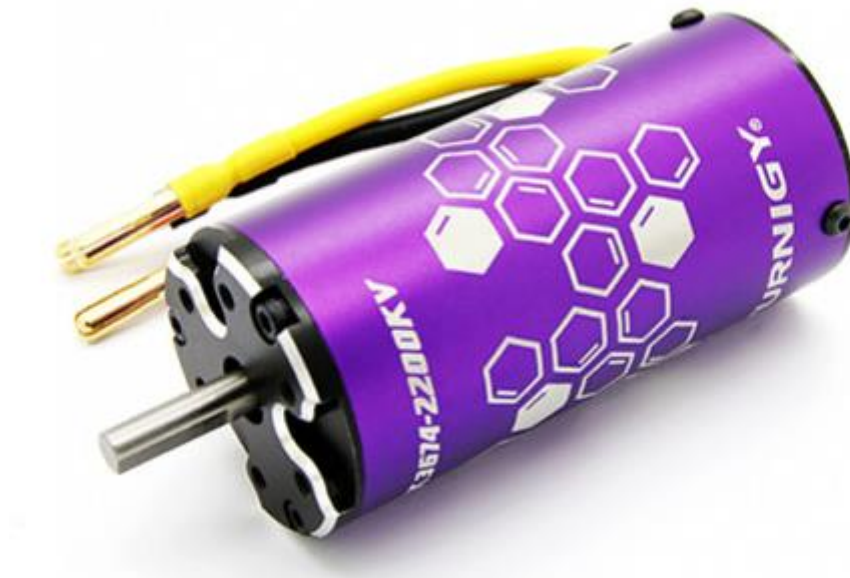
Figure 4.13. Turnigy XK3674-2200KV 1750w BLDC Inrunner Motor (source: hobbyking.com)
